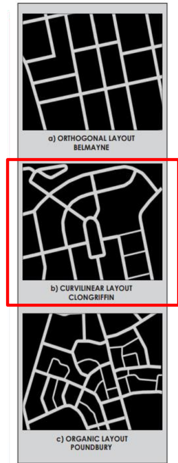
Figure 3.8: Permeable street layouts may be formed via a number of different configurations including examples of the more rigid orthogonal, curvilinear and/or organic.
